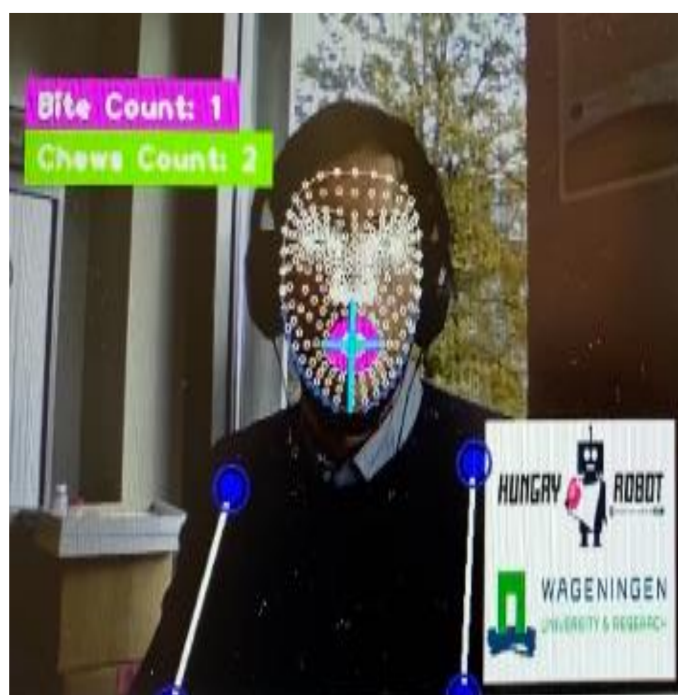
Figure 1. The 468 facial keypoints (white) are applied on a face. The lips contour (pink) and their distance (light blue) are highlighted.
