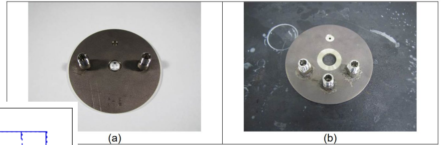
Top plates for prototypes after feedthroughs installed: (a) 1-2 and (b) 1-3.
