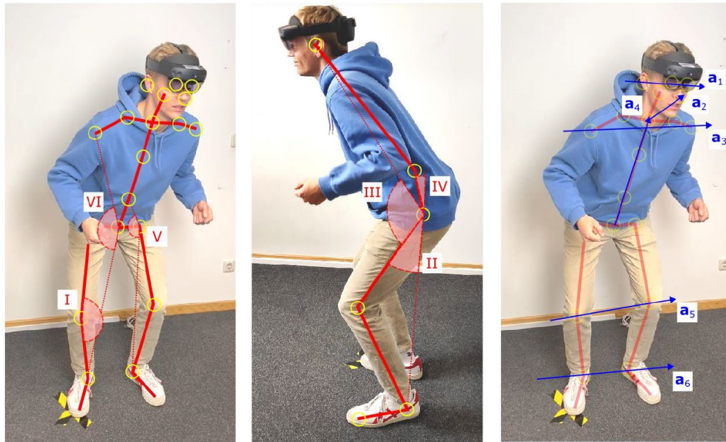
Figure 2. Example of body model with highlighted body nodes (yellow circles), body segments (red solid lines), body angles (I-VII), and body axes (blue vectors, a_i ). The first body angle (I) is defined from the triangle spanned between the knee, hip, and ankle.
