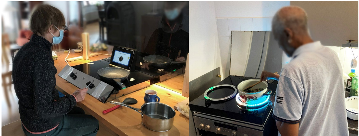
Figure 4. Wizard of Oz user testing with Cook3r prototypes (left: the Step-by-Step Cooking Prototype 2021 and right: the Routine-Based Cooking Prototype 2022)
