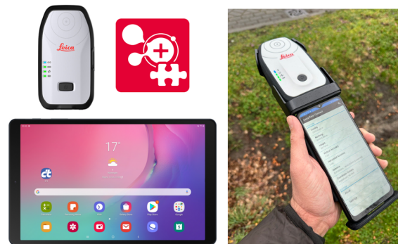
Figure 1. The hardware setup of the measurement system. The system includes a GNSS receiver (Leica FLX100+), a smartphone or tablet, and the Zeno Connect app.
