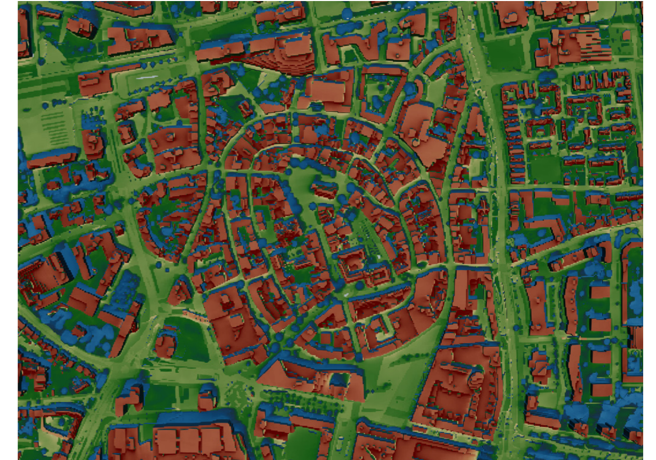
Surface Temperature for Control case: Roof albedo:0.1; Façade albedo:0.25
